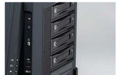
Multiple open bays
