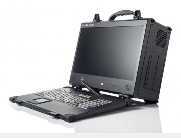
Compact, Rugged Portable with a 17.3" display and 4 full-length expansion slots. Configurable with the latest Intel® Core™ or AMD processor.
